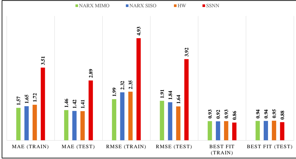
Figure 12: Statistical measures for training and validation of heating value.
